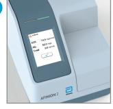
Record the result when it appears on the screen. Touch to accept. The lid opens automatically.
