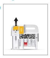
Pull the sampling device straight up from the test cartridge.
