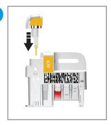
Replace the sampling device immediately. Analysis of the test cartridge must start within 1 minute.
