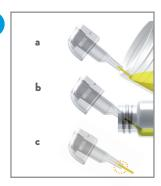
Fill the capillary; touch the surface of the patient sample (a) or control (b). Fill it completely (c). Do not wipe off the capillary.
